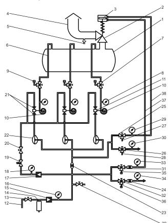
Control unit for controlling 1 safety valve does not contain these positions: 26, 28, 30, 32, 34, 36 a D, E, L, M.
